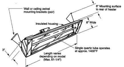
Wall/ ceiling brackets are furnished with all heaters. Their use is optional. When used, they allow heater to be fastened to wall or ceiling and then tipped up to 60°.
