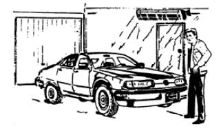
Install fixture to heat the area from the "cold side" if possible. This helps compensate for increased body heat losses due to exposure. Warm floors reradiate heat. Warmer air rises from floor. Some heat reflects from floor. Mounting a heater directly over a table or other obstruction will block the energy, primarily heating the object. It is best to move heater to the side, allowing complete body and floor coverage.
