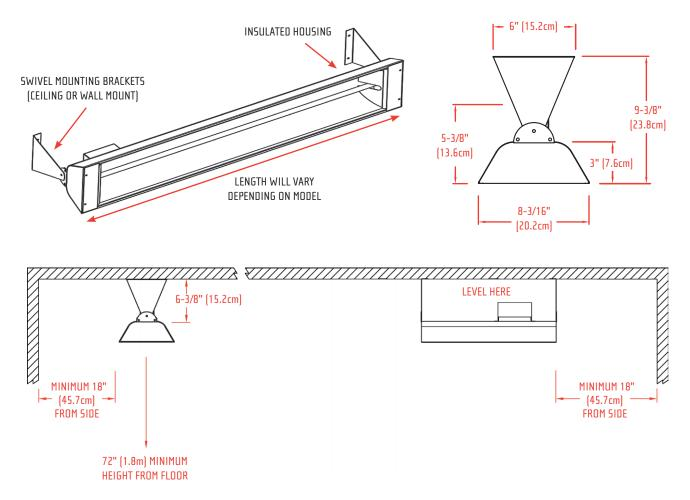
Heater must be installed with the quartz tube horizontally level. For maximum tube life, use a carpenter's level tool to find the optimum level position for the heater's body. Always maintain the minimum clearances from the heater body to any combustible materials.
