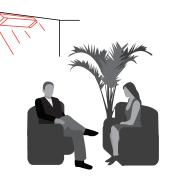
Install fixture to heat the area from the "cold side" if possible. This helps compensate for increased body heat losses due to exposure. Warm floors reradiate heat. Warmer air rises from floor. Some heat reflects from floor. Mounting a heater directly over a table or other obstruction will block the energy, primarily heating the object. It is best to move heater to the side, allowing complete body and floor coverage.
