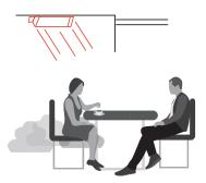
When outdoors, hang heater under protective roof or weather cover whenever possible. Even though heater is all-weather construction, it will last longer and look better if it is protected from rain and snow.
