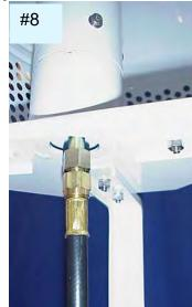
12. Remove the second protective plastic cap from the 3/8" flared fitting exiting the bottom of the post. Gently engage the fitting at the end of the hose/regulator assembly onto end of the fuel feed line being careful not to cross-thread the fitting. (See # 8) The swivel fitting at the end of the hose
