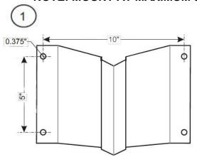
USE BRACKET AS TEMPLATE FOR HOLES/BOLTS TO THE STRUCTURE. FASTEN TO STRUCTURAL MEMBER[S] OR DEVISE STRUCTURAL SUPPORT TO CARRY WEIGHT OF HEATER AND WIND/ SNOW LOADS
