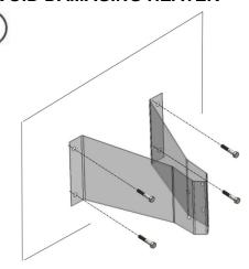
FASTEN WALL BRACKET TO STRUCTURE USING FIELD SUP-PLIED FASTENING HARDWARE. ENSURE SUFFICIENT STRENGTH AND INTEGRITY TOCARRYY WEIGHT OF HEATER AND WIND/ SNOW LOADS
