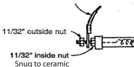
Use a thin 11/32" wrench to hold inside nut. Nuts must make a tight connection.
