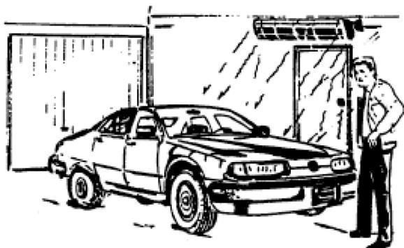
Install fixture to heat the area from the "cold side" if possible. This helps compensate for increased body heat losses due to exposure.
