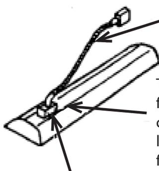
Connect power with flexible conduit or appropriate cord to allow heater to be swiveled.
