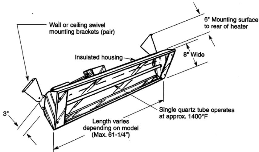
Wall/ ceiling brackets are furnished with all heaters. Their use is optional. When used, they allow heater to be fastened to wall or ceiling and then tipped up to 60°.
