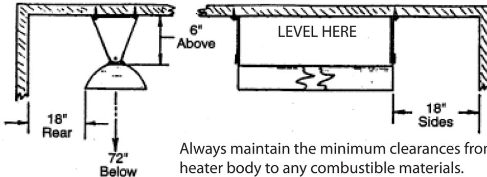
Always maintain the minimum clearances from the heater body to any combustible materials.
