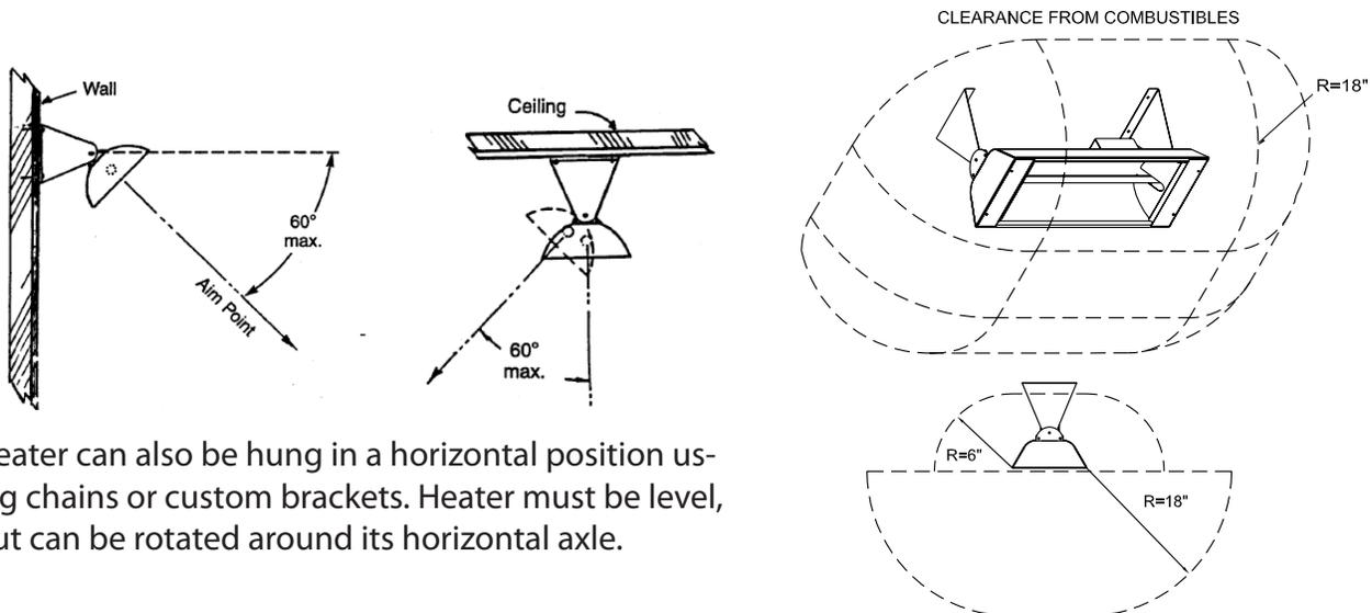
Heater can also be hung in a horizontal position using chains or custom brackets. Heater must be level, but can be rotated around its horizontal axle.
