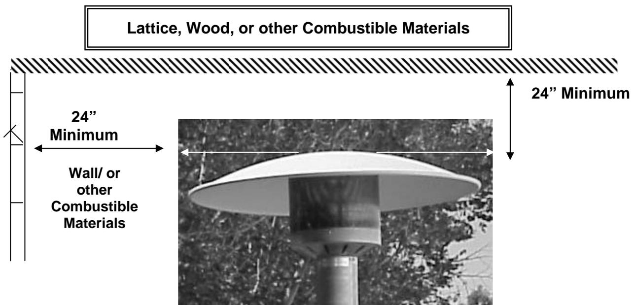
These minimum clearances from combustible materials must be maintained anytime the heater is in operation. **We recommend the heater shall have clear opening from the top of the reflector.**
