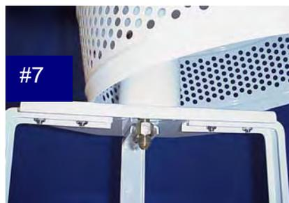
If you use both flat and locking washers at this connection the sleeve will not be able to slide over the fasteners.
