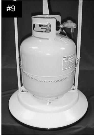
(See #9) If you are sure that the fittings at the end of the feed line going into the burner head and the other end of the fuel feed line where the hose is attached are tight turn on the fuel at the cylinder and test these two connections one at a time with a soapy solution. You will need to lift heater head out post to check this
